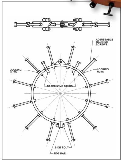
The PLIDCO<sup>®</sup> Ovality+Gauge is designed to accurately measure the outside surface of a pipe, particularly during limited conditions of reduced visibility underwater. A circular cross section, free of any indentations or flat spots that would adversely affect the sealing properties of a PLIDCO<sup>®</sup> repair fitting, can be confirmed using the PLIDCO<sup>®</sup> Ovality+Gauge.
